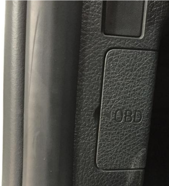
Picture1. OBD diagnosis socket of BMW 1 series
