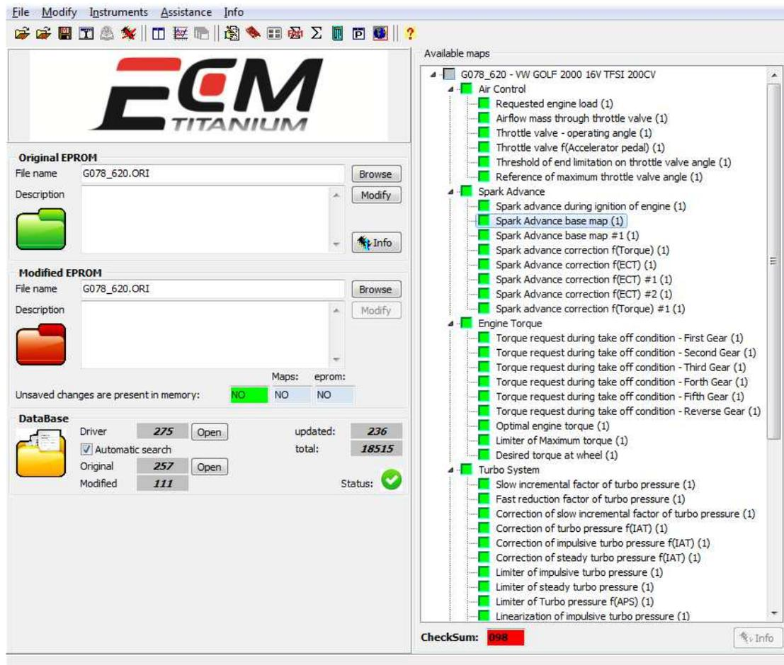
Picture 15: *ECM Titanium* main window; file with *associated Driver*.
