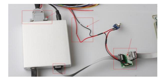
When you connect ECU BDM cable, please pay attention do it correctly, and the color of the cable should be not mistaken.
